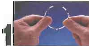
1 Fitter compresses Gap-A-Let® ring to fit into pipe fitting.
