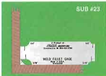
SPECIAL FILLET GAUGE LEG LENGTH ONLY
