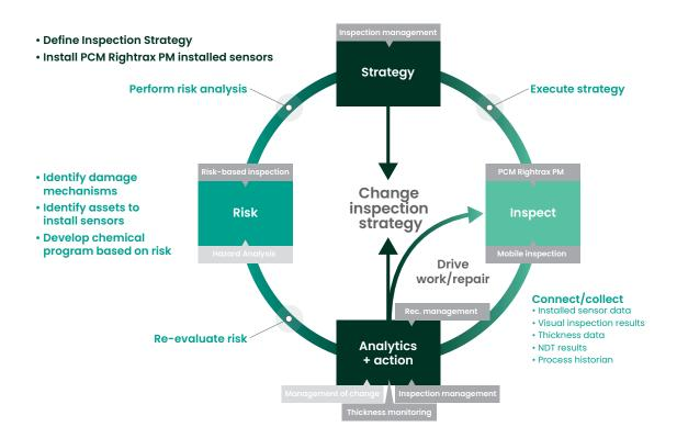
Waygate Technologies' PCM solution enhances the Intelligent Asset Strategy cycle. Traditionally, organizations utilize Risk-based Inspections (RBI) tools and follow the Intelligent Asset Strategy cycle to drive their inspection programs and support reliable operations. With PCM, operators can introduce permanently installed sensors on critical assets to monitor in near real-time the wall loss and corrosion rate, enabling them to take a proactive approach to manage the risk of corrosion.
