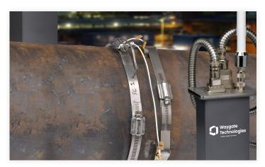
Sensors are affixed to a pipe or other surface by bands and a dry couplant expected to last indefinitely. However, should you need to remove them, the sensors can be detached with no hot work or damage to the asset.
