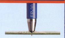
The hand-held ITM-525 is the enhanced successor to the ITM-52 model designed for fast, precise, non-destructive measurement of copper thickness in plated through-holes and copper laminate of unetched printed-circuit boards (PCB). ITM-525 is used for in-process control to maintain high-quality PCB production. It is battery powered and equipped with an internal charger.
