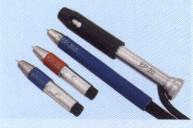
The ITM-525 consists of a basic unit offering a variety of probe sizes. Eddy current probes for through-holes are detachable, consisting of a probe holder with replaceable EP-25 and EP-30 plug-in cartridges. The EP-20 probe is not detachable. Probe tips\* are inserted into through-holes to take readings. Due to the special construction of probe tips, cracks in the copper can be detected. Shortened probes EP-25S and EP-30S are available.
